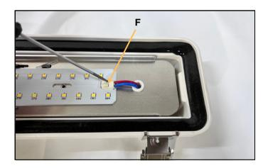
Once the buttons are pressed, gently pull the wires away from the driver to fully disconnect them. Take note of the wire locations for easier reinstallation later.
