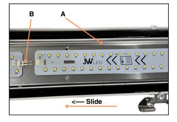
**2.** Next, re-attach the positive and negative wires to the new LED board.
