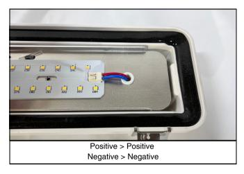
**3.** Using the 3 removed screws **(C)** from earlier, secure the new LED board to the mounting plate.
